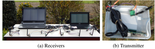
Figure 2: The experimental setup with seven SX1276 devices interfaced with Arduino Pro Minis.
