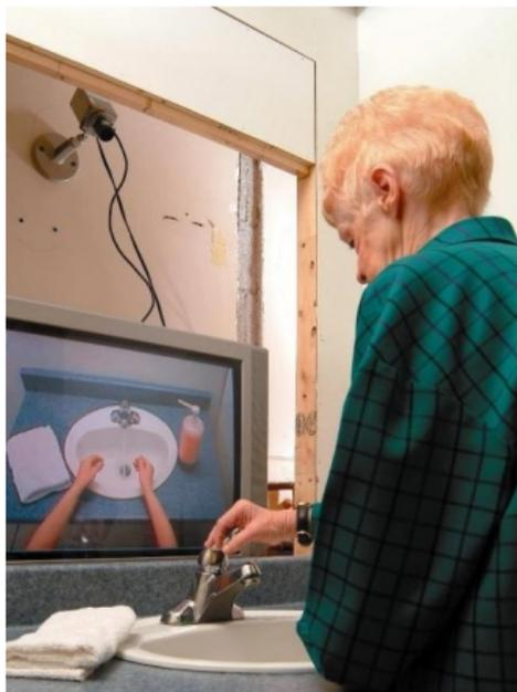
An intelligent cognitive device that tracks a user through handwashing, providing cues when necessary.
